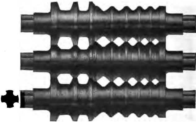
FIG. 117.—Roughing rolls for making bars for shrapnel. ( Courtesy of Scientific American. )
